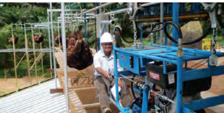
Mechanised crop evacuation being tested at Lavang Estate, Sarawak
